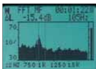
FFT narrow band spectrum (option HD2110.06)
