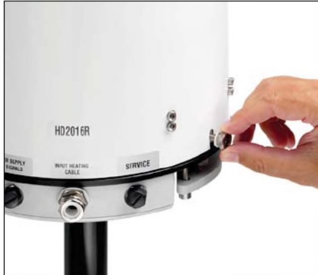
Sequence to remove the cylindrical cover from the base of the rain gauge.
