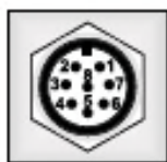
Instrument M12 male connector
